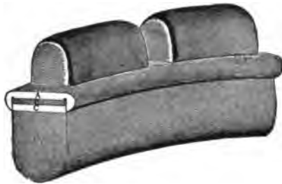
FIG. 95.—Solid Rubber "Sectional Tire," having the tread divided into a number of tooth-like sections, all attached in one piece to the rubber base, as shown, in order to give greater distortion endwise under load, thus allowing of considerable cushion effect. It has been claimed that the construction permits of real resiliency.
